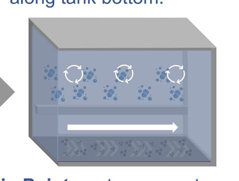
**Bucklin Point:** vortex separator removes grit like a centrifuge.
